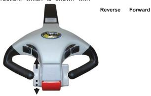
The degree of rotation determines the speed of movement, so the farther you press the wheel in either direction, the faster the S3 will travel, up to a maximum speed of ~3mph when unloaded or ~2.6mph when loaded to capacity. Simply by releasing the movement control, the S3 will decelerate to a complete stop.
